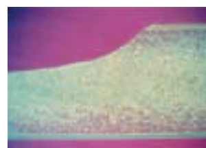
DELIN® 500 after wear test (test specimen).
