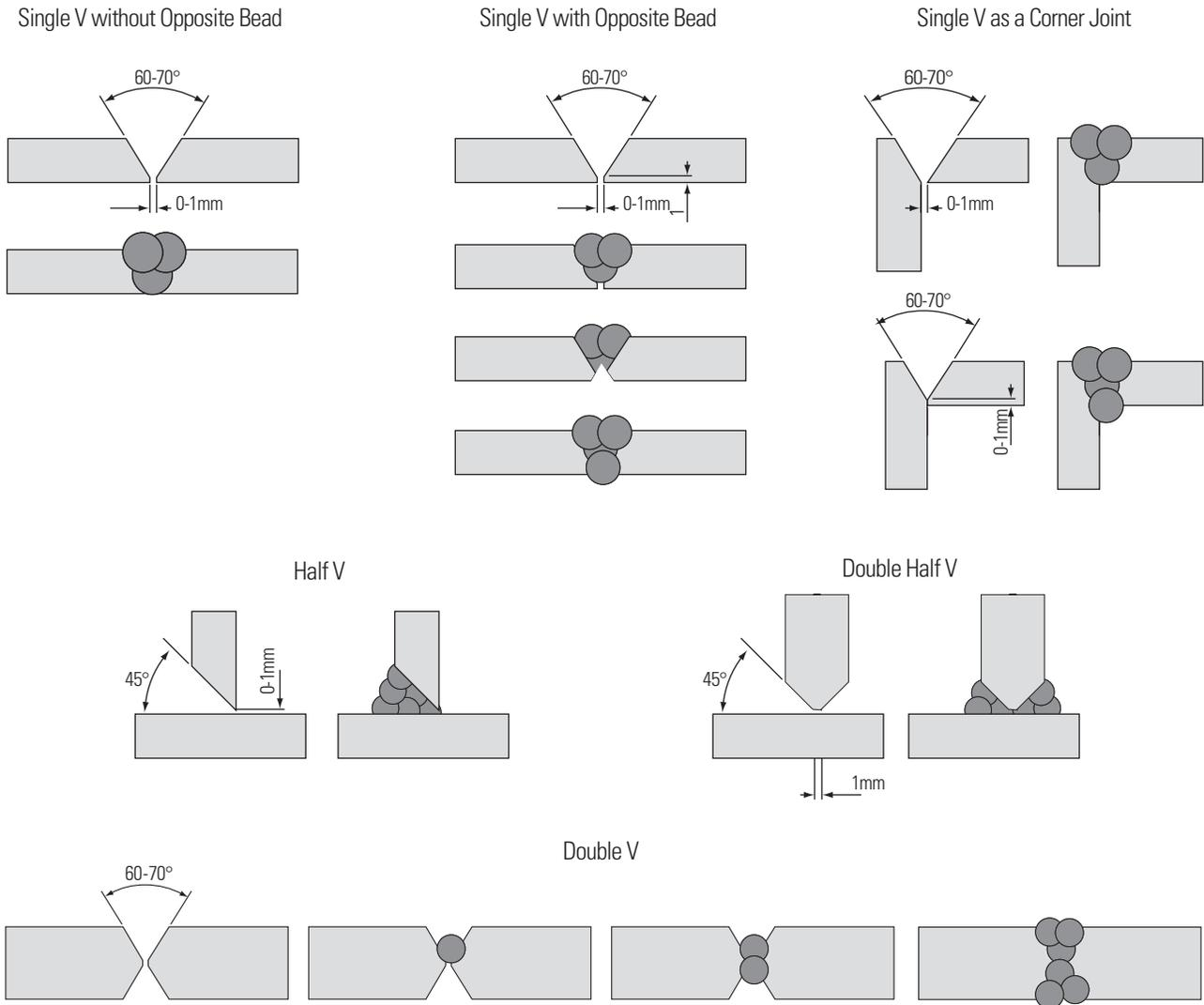
**Figure 3: Typical Welded Joint Configuration**
